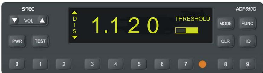
**Fig. 2-14. Threshold Function**
