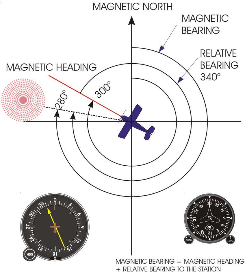
**Fig. 3-5. Determining Magnetic Bearing Using DG**
