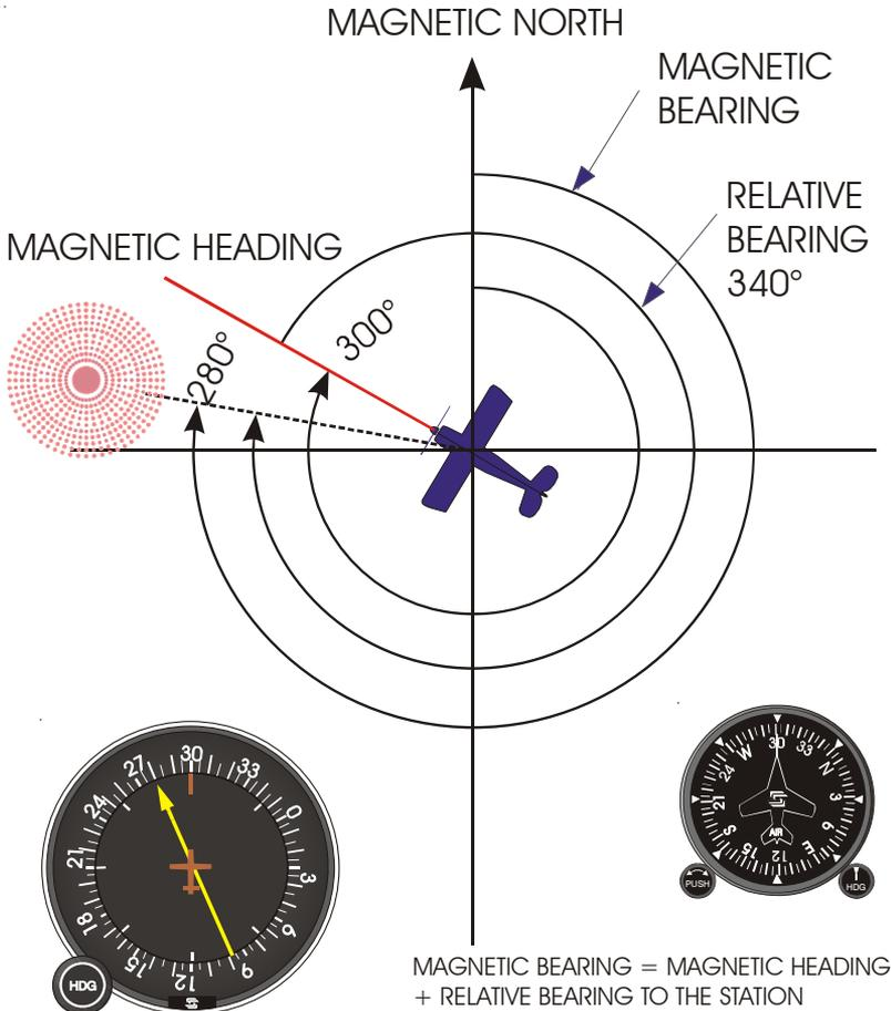
**Fig. 3-6. Determining Magnetic Bearing Using HDG Knob**
