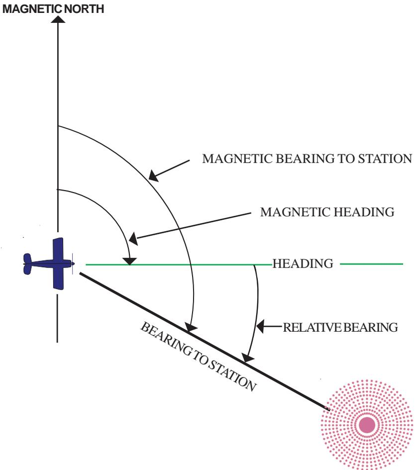
**Fig. 3-4. Relative and Magnetic Bearing**
